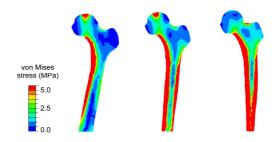
Fig.1: Stress distribution (-2sd, average and +2sd) corresponding to a load applied on the head.
