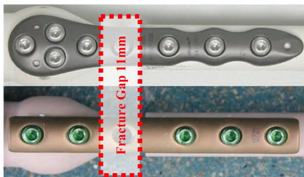
Fig. (3). Implants chosen in the biomechanical testing, top: novel VariAx Plate, bottom: 1/3 Tubular LC Plate.
