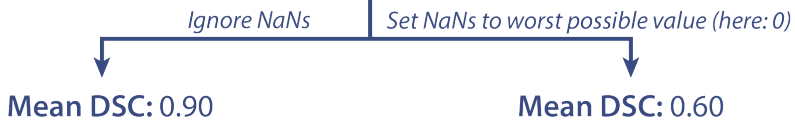
Fig. 38. Effect of invalid predictions (missing values) when aggregating metric values. In this example, ignoring missing values leads to a substantially higher Dice Similarity Coefficient (DSC) compared to setting missing values to the worst possible value (here: 0).
