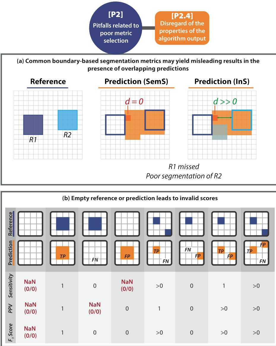
Fig. 8. [P2.4] Disregard of the properties of the algorithm output. (a) Possibility of overlapping predictions. If multiple structures of the same type can be seen within the same image (here: reference objects R1 and R2 ), it is generally advisable to phrase the problem as instance segmentation (InS; right) rather than semantic segmentation (SemS; left). This way, issues with boundary-based metrics resulting from comparing a given structure boundary to the boundary of the wrong instance in the reference can be avoided. In the provided example, the distance of the red boundary pixel to the reference, as measured by a boundary-based metric in SemS problems, would be zero, because different instances of the same structure cannot be distinguished. This problem is overcome by phrasing the problem as InS. In this case, (only) the boundary of the matched instance (here: R2 ) is considered for distance computation. (b) Possibility of empty prediction or reference. Each column represents a potential scenario for per-image validation of objects, categorized by whether True Positives (TPs), False Negatives (FNs), and False Positives (FPs) are present ( n > 0 ) or not ( n = 0 ) after matching/assignment. The sketches on the top showcase each scenario when setting " n > 0 " to " n = 1 ". For each scenario, Sensitivity, Positive Predictive Value (PPV), and the F_1 Score are calculated. Some scenarios yield undefined values (Not a Number (NaN)).
