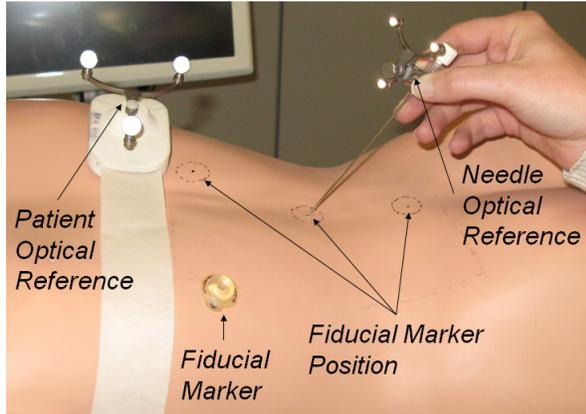
Fig. 2. Patient optical reference setup with the fiducial marker used for imaging and their respective positions marked with a surgical pen.
